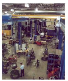
are no less than 57 single and twin-hoist overhead cranes, eight jib cranes and 29 monorail hoists. The overhead units provide spans of up to 19,400mm and safe working loads (SWL) up to 4000kg (the huge jet engines are broken into sections for overhaul and repair work to be carried out), while the jib cranes — both underbraced and overbraced floor-mounted types — offer SWL up to 1000kg and jib arm lengths up to 3500mm.
